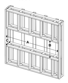
CAUTION: This fireplace is NOT load-bearing. Ensure the opening for the fireplace is framed in such a way that the weight of the building materials will not create pressure on the top of
