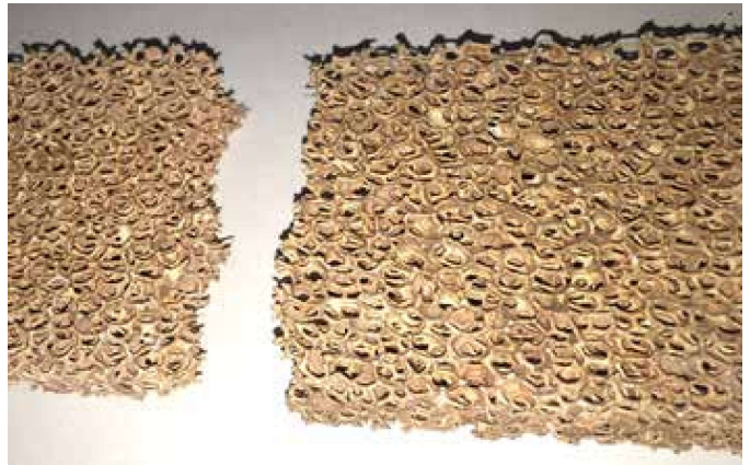
Combustor Problem - Broken Combustor
