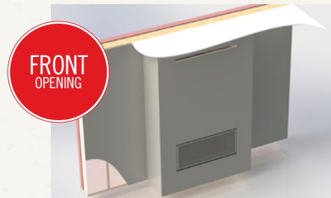
Uses an air outlet opening that will be built into the front of the constructed enclosure, at the top, centered above the appliance.
