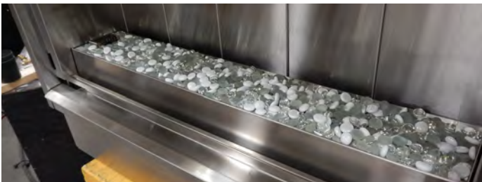
Figure 66 Spreading the firestones evenly and make sure there are no firestones covering the pilot.
