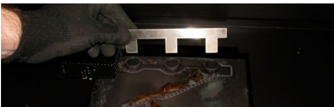
Figure 23.d Pushing the Rock Guard down into place.
