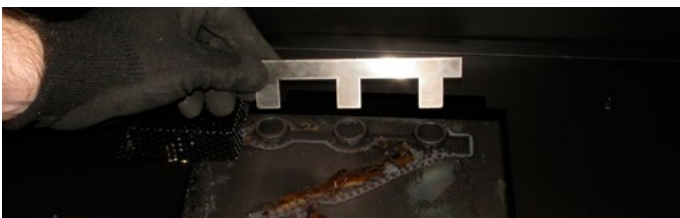
Figure 23.c Pushing the Rock Guard down into place.
