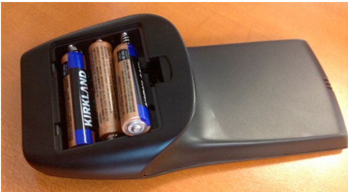
Figure 27.d Remote Control Battery Compartment
