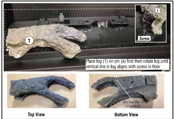
Figure 48 - Place front left log (1)
