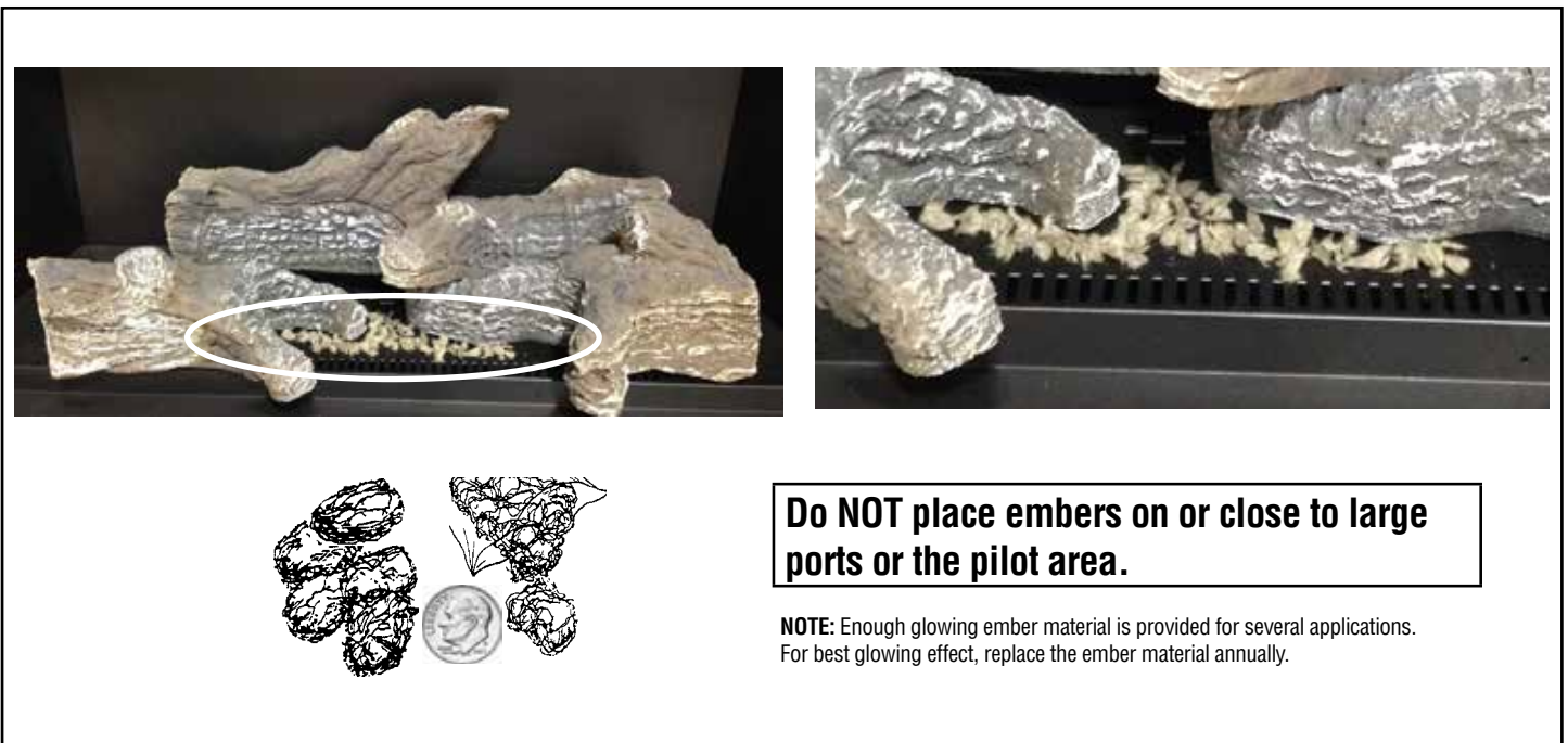
Figure 60 - Place glowing embers (rockwool)
