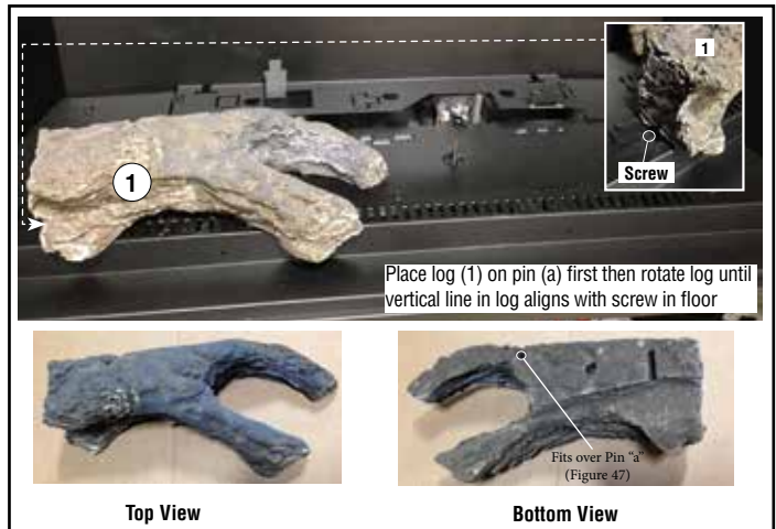
Figure 48 - Place front left log (1)
