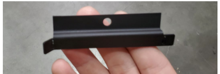
Figure 20.b Bend the left side tab
