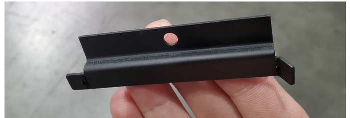
Figure 20.b Bend the right side tab
