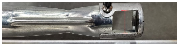
Figure 13.c primary air adjuster
