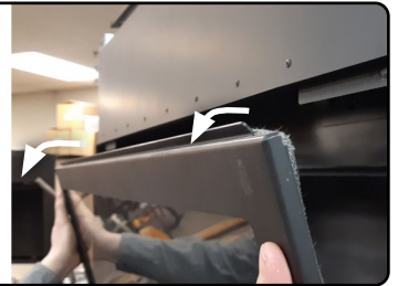
Figure 21.e Lift the door
