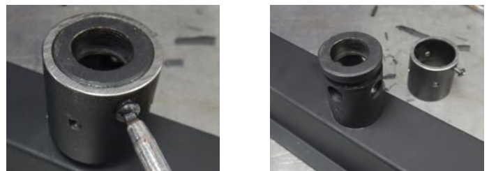
Figure 13.c Removing the orifice
