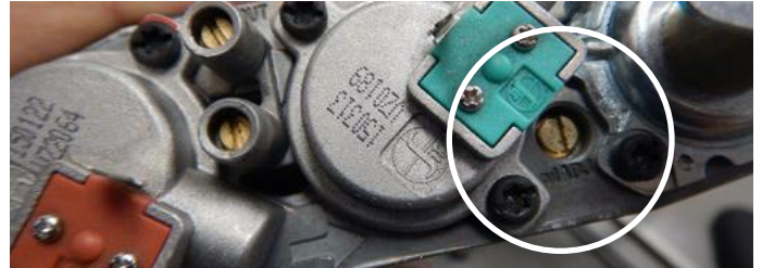
Figure 13.g Adjust pilot size
