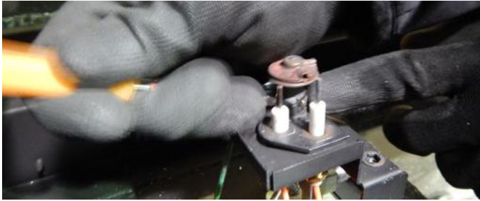
Figure 13.d Removing the spring clip
