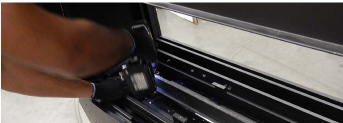
Figure 12.d Removing the Burner screws
