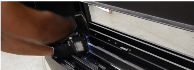
Figure 12.d Removing the Burner screws
