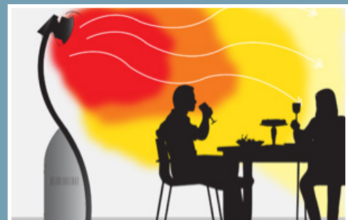
Directional heat implies that the majority of the heat produced is pushed in one direction, allowing for better heat coverage.
