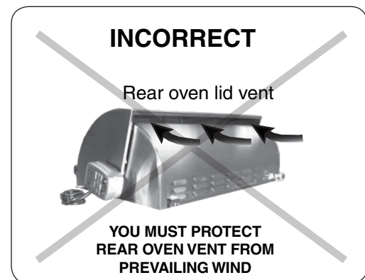
Fig. 12-3 Airflow direction - INCORRECT
