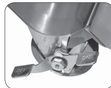
Fig. 3-3 Locking the casters
